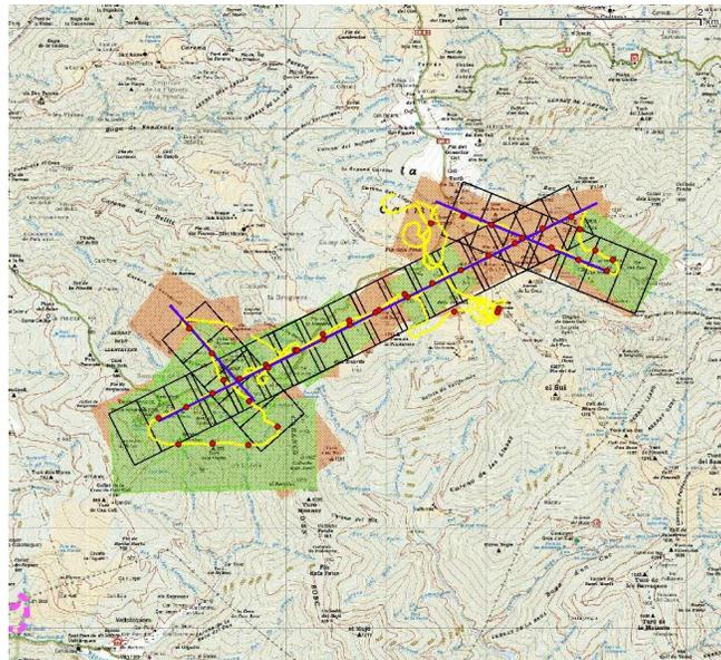
Figure 6. Example of a campaign conducted by the minUAV ATCOR-3. The blue lines and black rectangles are, respectively, the planned flight lines and image footprints (700 m agl). The yellow line and red dots represent, respectively, the GPS track and positions of image acquisitions. The orange and green areas represent the mosaic of estimated footprints of image acquisitions.
