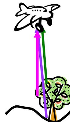
The scanning path (shape, spot diameter, distance between spots, n° of pulses per scanning line etc...) depends on the instrument used and on the flight height.
