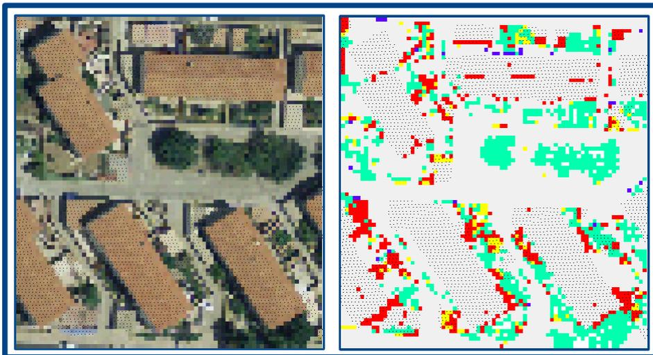
The Orthophoto is generated using a DTM → the building shapes are shifted proportionally to their heights.
