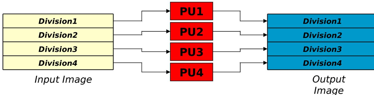
Tiling: combination of threading and streaming capabilities
