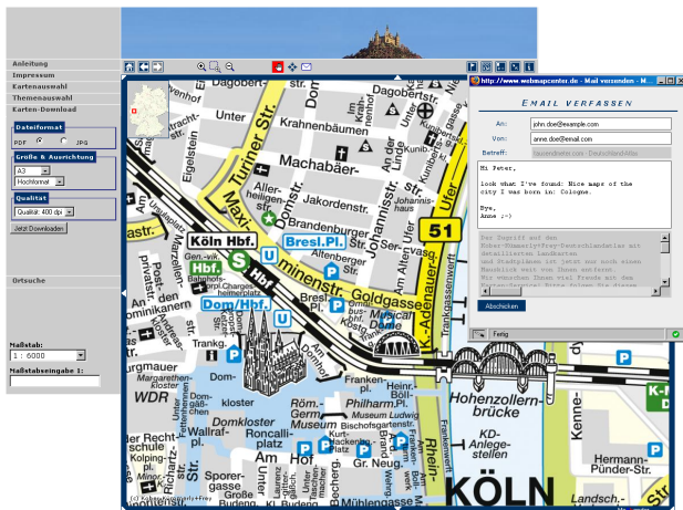
Figure 1: A demo application of Mapbender. Notice the toolbar (top), Menus (left, visible: PDF-options) and the email-dialog to send a link of the current extent (upper right corner). Image copyright: Kober-Ki&#x2013;immerly+Freya Media AG, Cologne, Germany. Used by permission.
