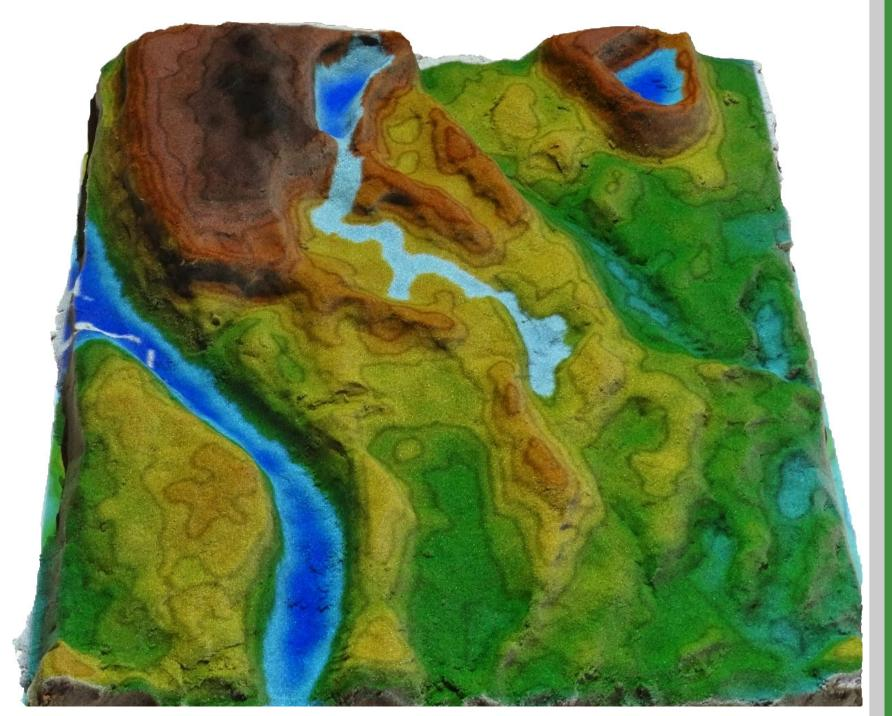
Coal ash pond breach in Tangible Landscape environment using *r.damflood* module
