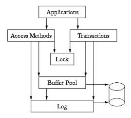
In this model, the application makes calls to the access methods and to the Transaction subsystem. The access methods and Transaction subsystems in turn make calls into the Memory Pool, Locking and Logging subsystems on behalf of the application.
