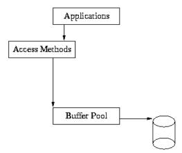
As you can see from this diagram, the application makes calls into the access methods, and the access methods use the underlying shared memory buffer cache to hold recently used file pages in main memory.
