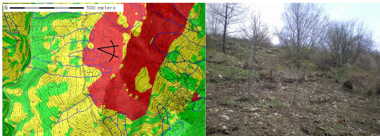
Figure 4. Evidence of ground movements in a high hazard area (Landslide Inventory map in blue).
