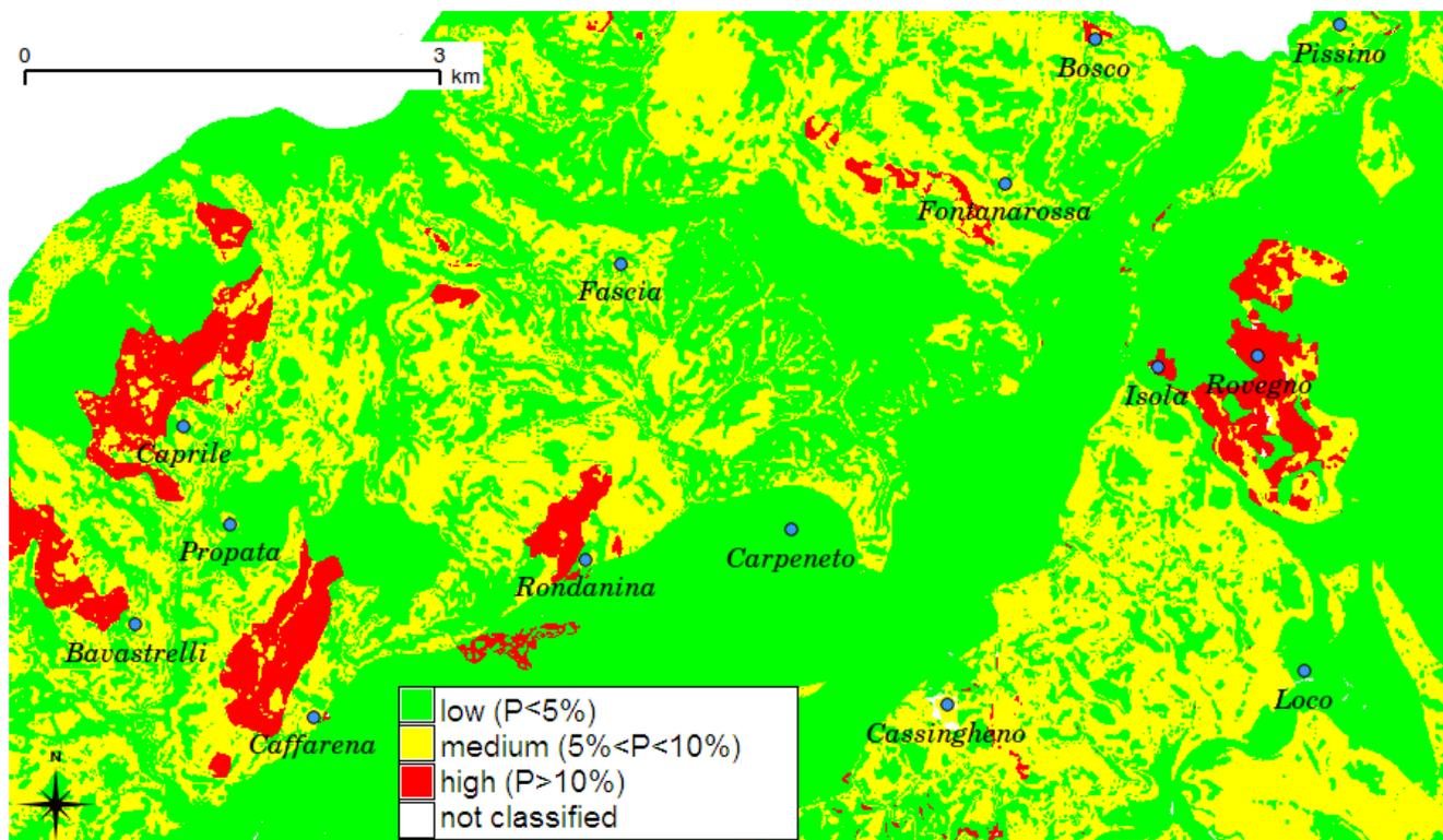
Figure 3. Landslide hazard map obtained for the study area.
