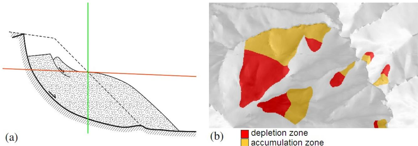
Figure 1. Division of a landslide in accumulation and depletion zones: (a) sketch of a ground profile, where the red line represents the ideal tangent line in the flex point of the slipped surface; (b) results of the proposed procedure.
