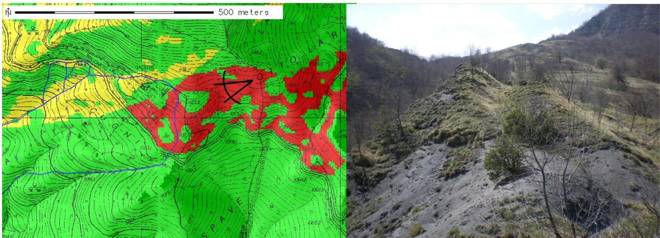
Figure 5. Evidence of ground movements in a high hazard area (Landslide Inventory map in blue).
