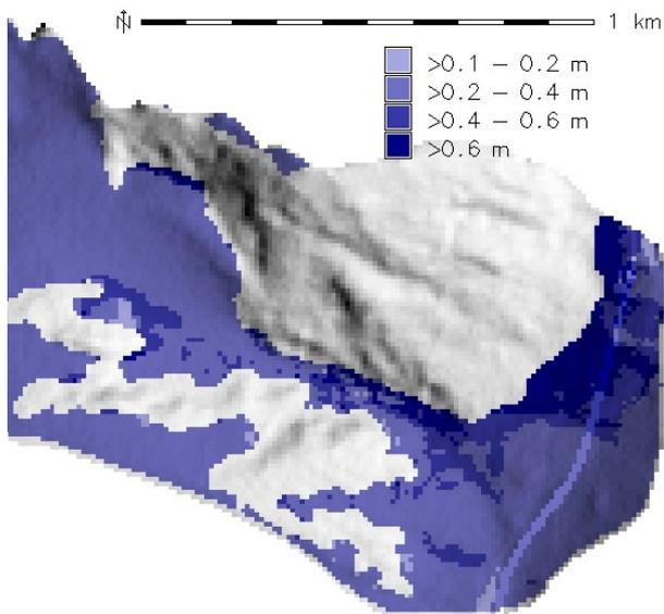
Figure 8: Maximum depth of saturation computed for 100 mm rainfall event.
