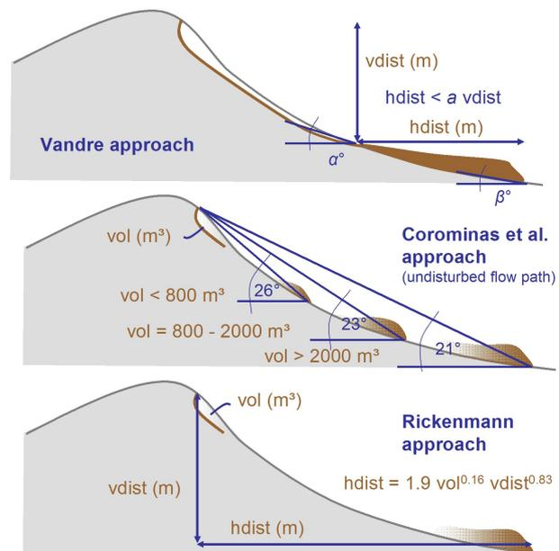
Figure 5: Runout models.
