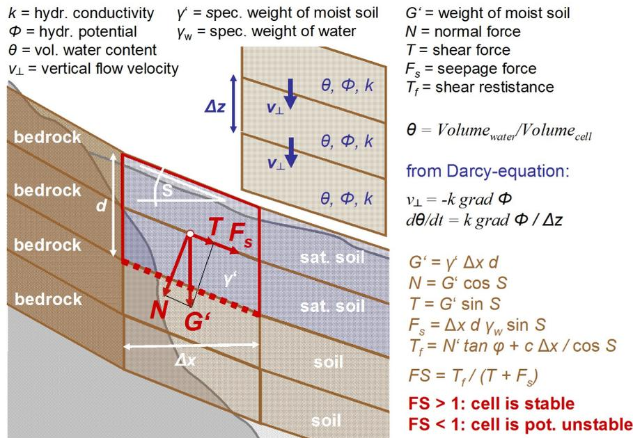
Figure 3: Subsurface hydrology and slope stability model.
